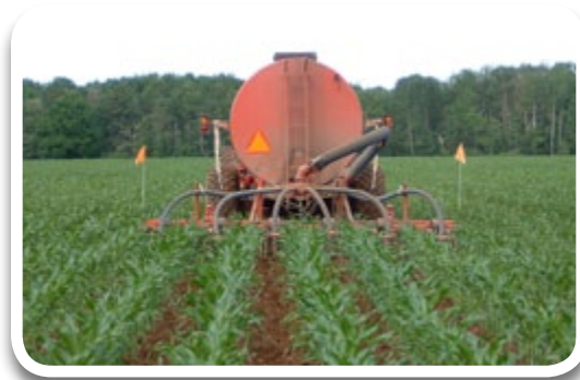
Manure application by injection
