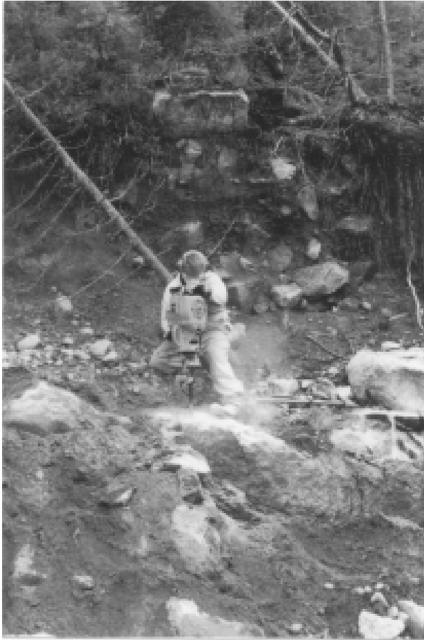
Figure 5. The primary method for collecting fresh samples involved use of a small gasoline-powered drill, wedges and feathers.
