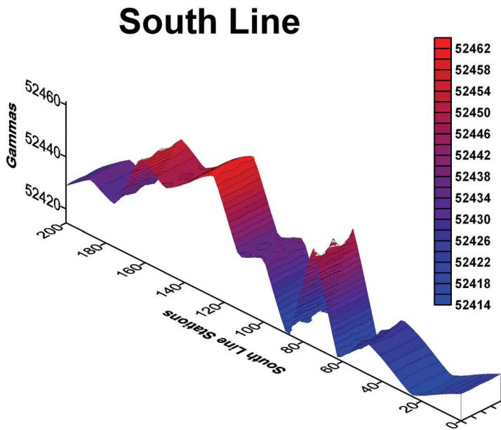
**Figure 7.** South line magnetometer signature for Gays River Zn-Pb deposit, Gays River, Halifax County, Nova Scotia.
