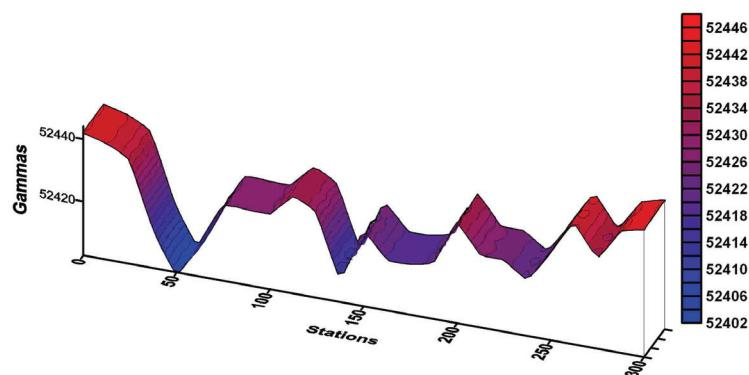
**Figure 8.** Fence line magnetometer signature for Gays River Zn-Pb deposit.
