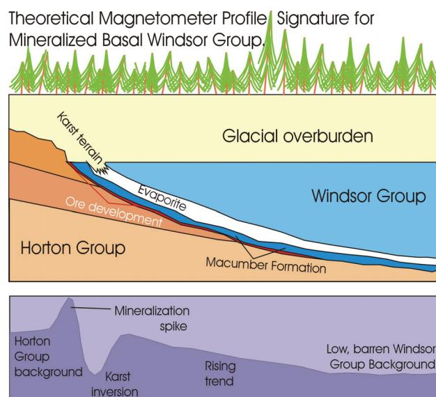
**Figure 2.** Theoretical magnetometer profile for mineralized basal Windsor Group.
