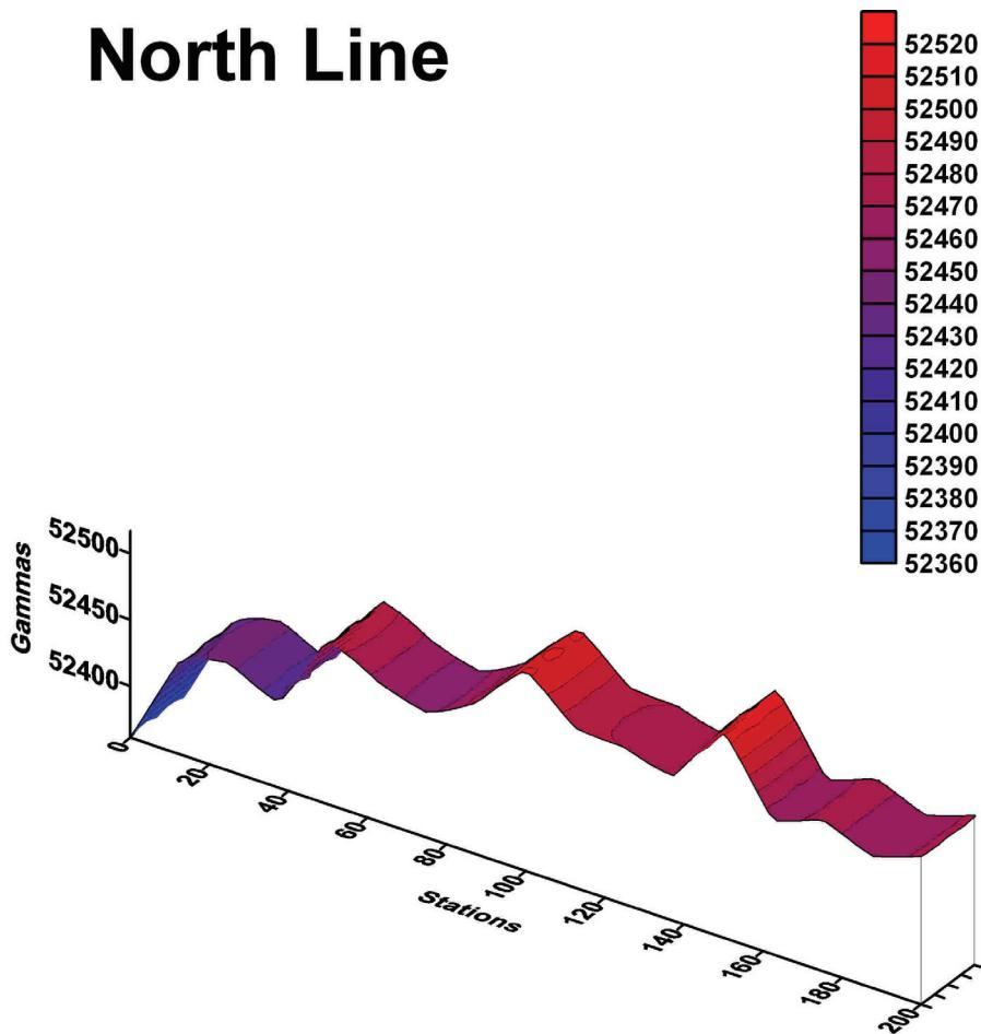
**Figure 9.** North line magnetometer signature for Gays River Zn-Pb deposit.
