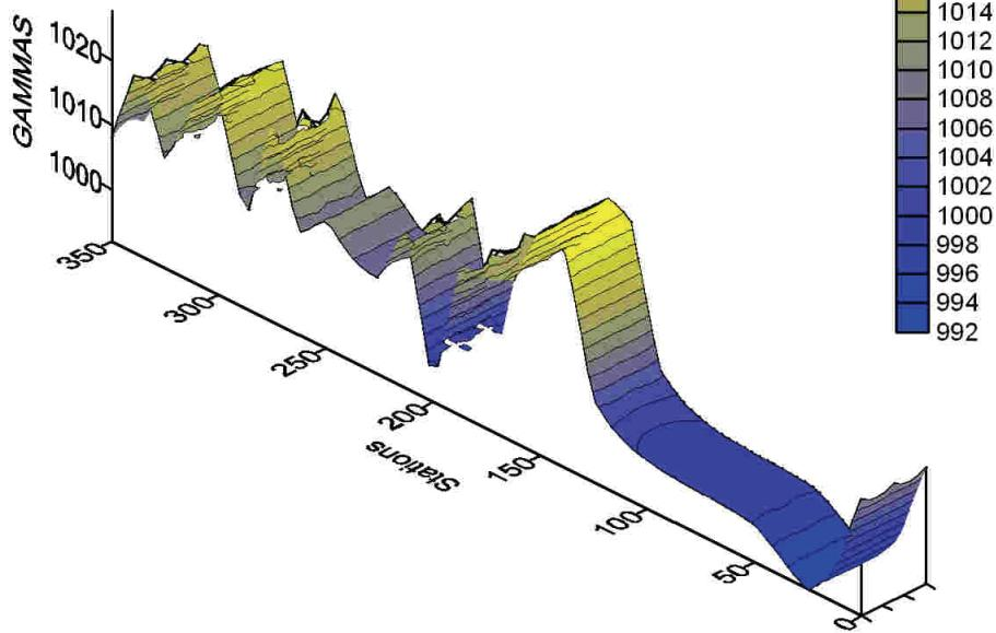
**Figure 5.** Signature exhibited at Tennycape on line surveyed with proton magnetometer.
