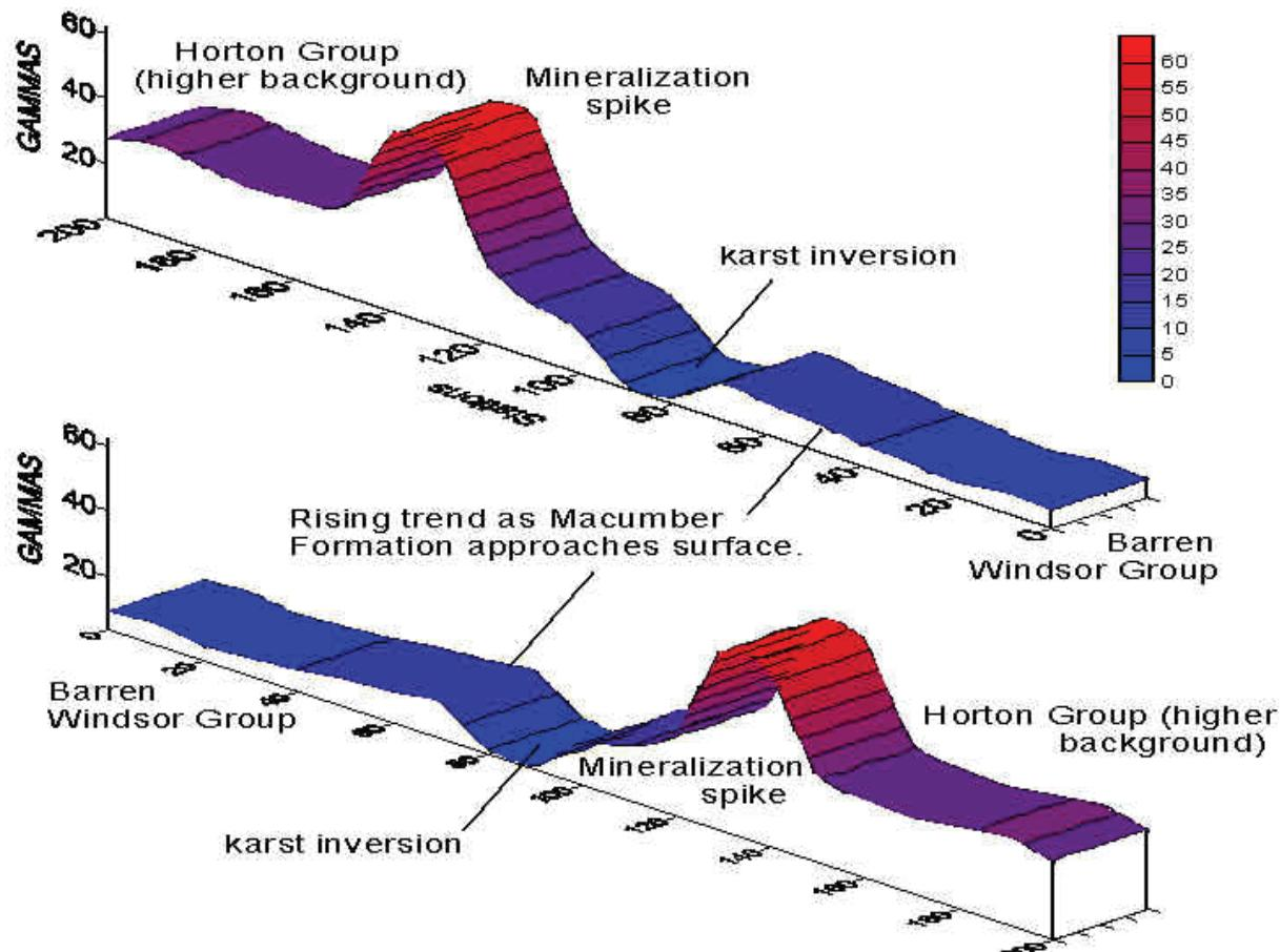
**Figure 3.** Expected signature to be encountered for the theoretical profile using a proton precession magnetometer.
