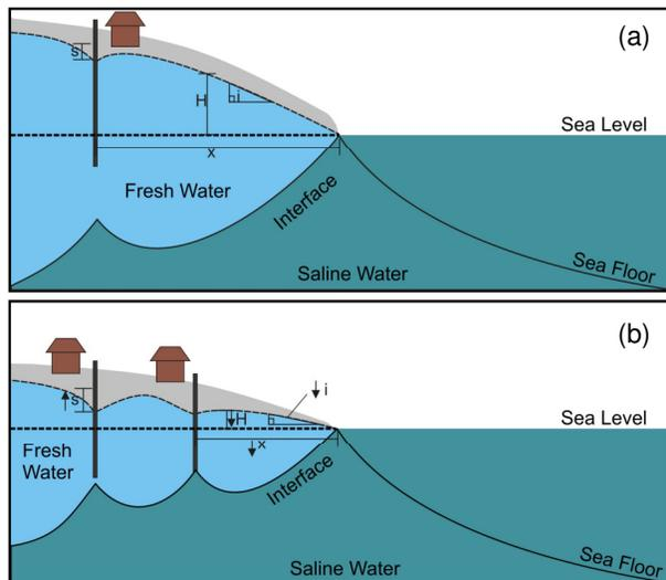
Figure 3. Conceptual illustration showing how vulnerability to SWI impacts can increase according to the Ghyben-Herzberg relationship. In (b), the water supply wells are at greater risk due to lower freshwater head above sea level ( $H$ ) as a consequence of their closer position to the coast, a lower hydraulic gradient ( $i$ ) and increased drawdown ( $s$ ).
