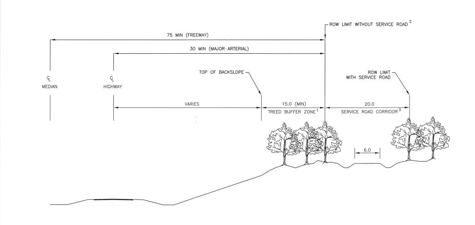
1. TO BE CONSIDERED WHEN A SERVICE ROAD IS REQUIRED IN CUT OR SHALLOW FILL AREAS, TO PREVENT DAMAGE TO CROPS, DRIFTING SNOW, ETC.
