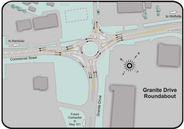
Modern roundabouts are specially designed intersections with traffic circulating around a central island. They have a proven track record around the world for reducing the number and severity of collisions and for keeping traffic moving smoothly.
