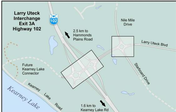
Modern roundabouts are specially designed intersections with traffic circulating around a central island. They have a proven track record around the world for reducing the number and severity of collisions and for keeping traffic moving smoothly.
