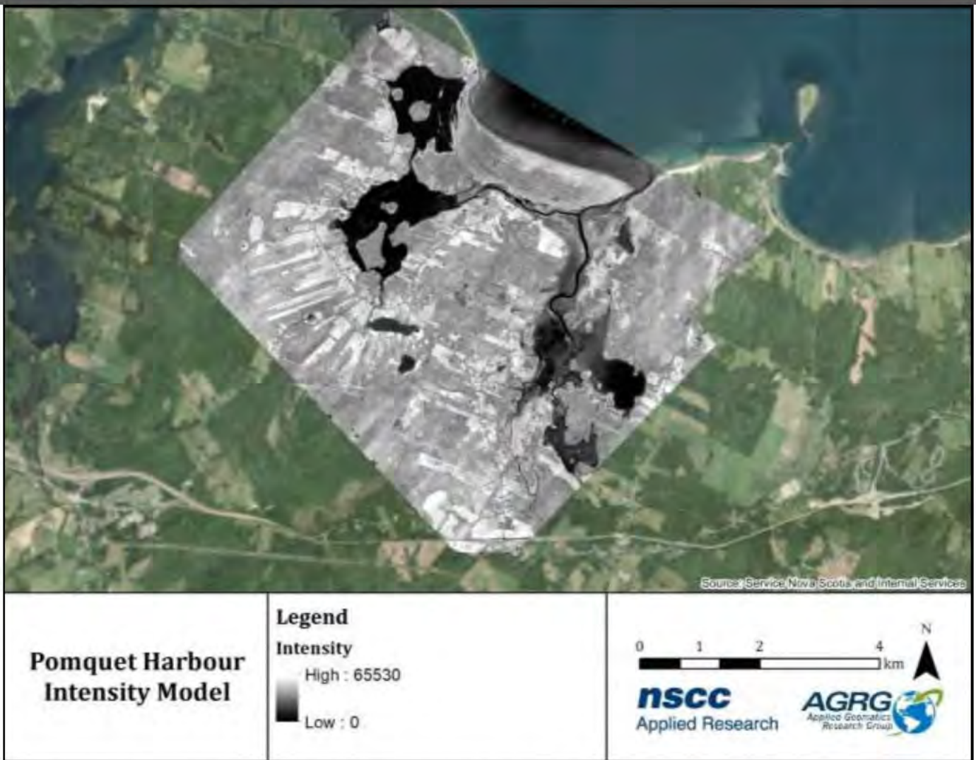
Figure 46: Intensity map of the lidar return data that incorporates all green laser returns above and below the water line (HHWL).
