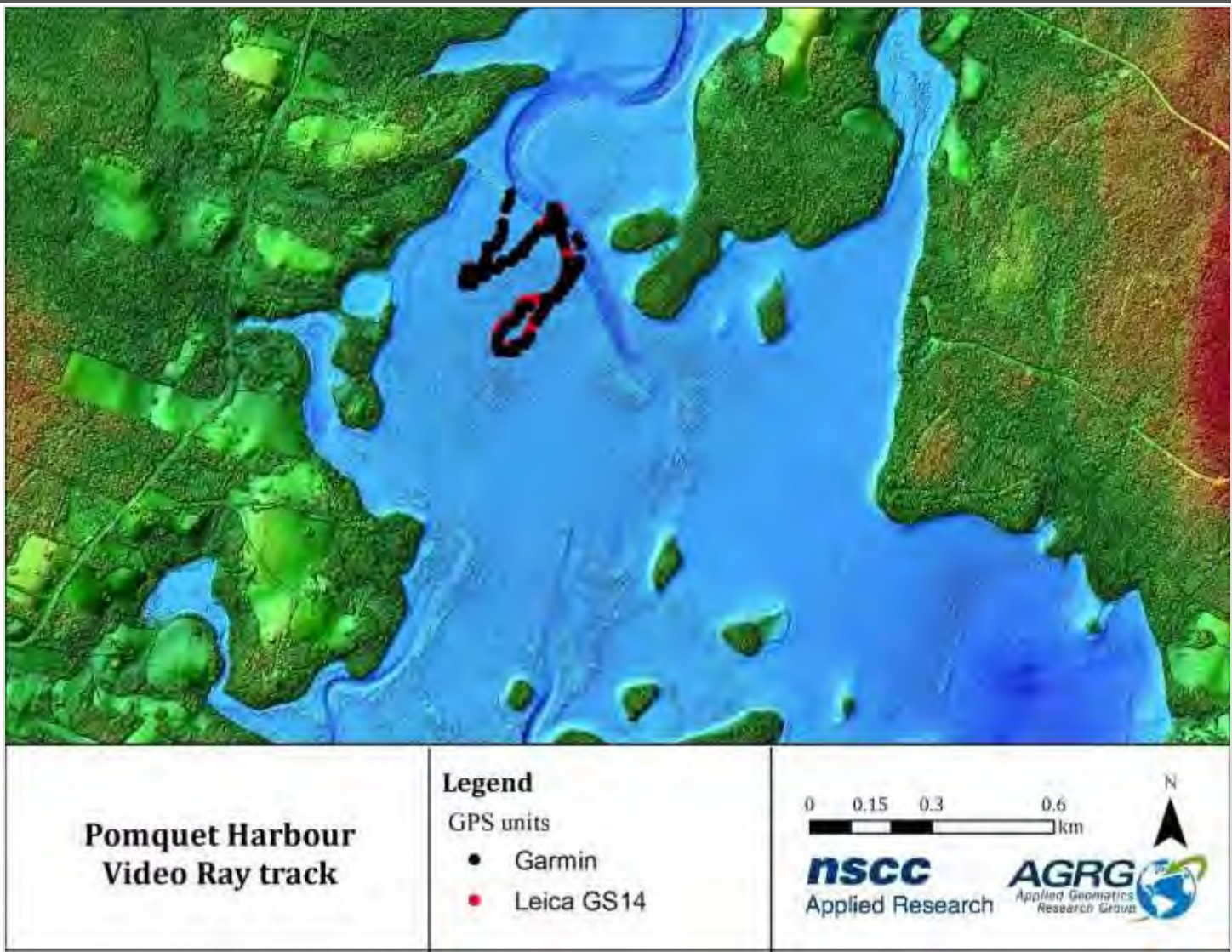
Figure 10: Video ray track obtained from the GPS units Garmin (autonomous >5 m accuracy) and Leica GS 14 (RTK corrections < 0.05 m accuracy) overlaid on a CSR.
