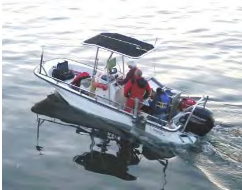
Figure 5: AGRG Boston Whaler with deployed multibeam system on an arm that rotates to submerge the echo sounder.
