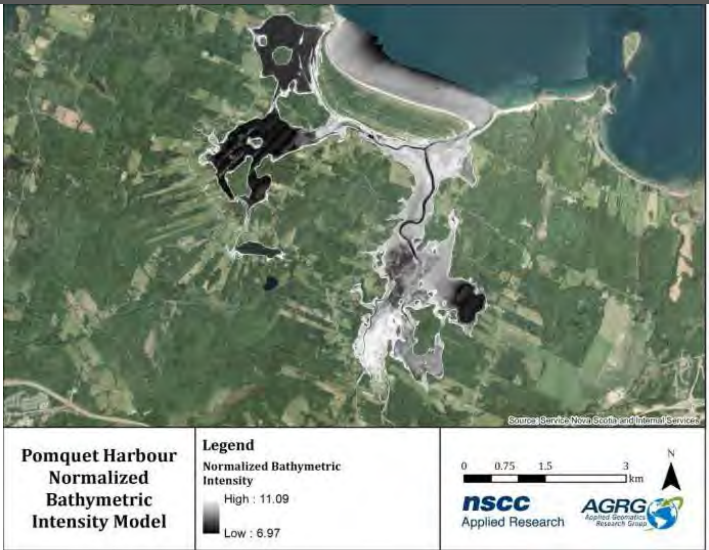
Figure 47: Normalized intensity map of the lidar return data that incorporates lidar returns below the water line (HHWLT).
