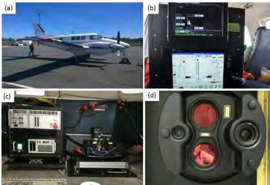
Figure 3: (a): Aircraft used for lidar survey; (b): display seen by lidar operator in-flight; (c): main body of sensor (left) and laser pointing through a hole cut in the bottom of the plane (right); (d): large red circles are the lasers; the RCD30 lens (right) and low-resolution camera (left).
