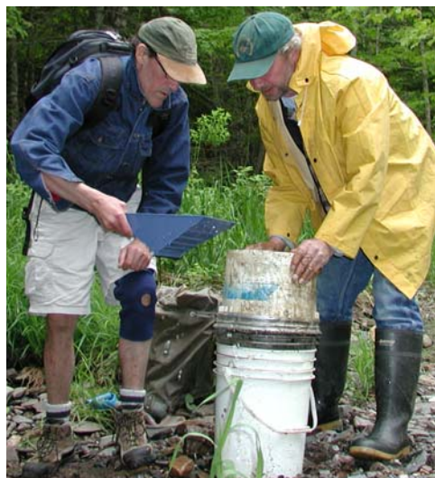
Brad Maynard (L) and Lindsay Allen, President of NSPA, process alluvium for placer gold.
