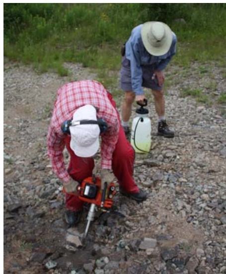
Dr. Laurie Brown (in red) drills in a bed of red sandstone in the Bears Brook Formation, trying to aim the hollow drill perpendicular to bedding. Dr. Christopher Condit (in blue) acts as field assistant, carrying a large plastic bottle of water and drilling fluid, which is pumped over the hollow drill bit continuously to prevent damage.
