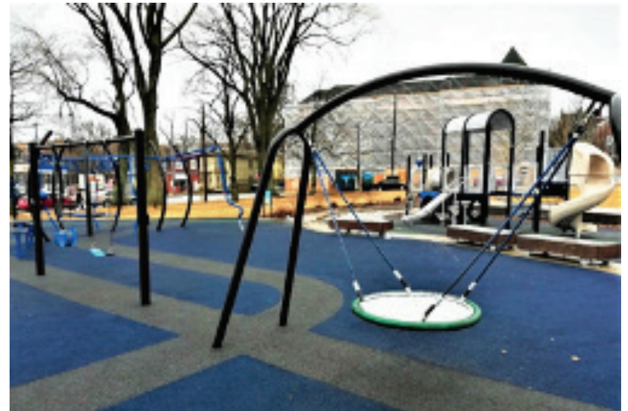
A playground surface able to absorb the shock of a fall (5.4.2.c) and containing a stand-alone feature (5.4.2.f)
