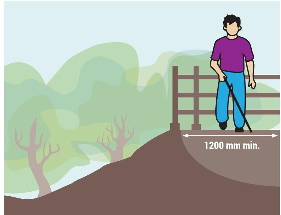
Wherever possible, pathways should have a width of 1200 mm or more, or provide passing space at that width frequently (5.4.1.d). Protective guardrails should be provided where there is a drop-off from the trail or pathway's edge (5.4.1.g).
