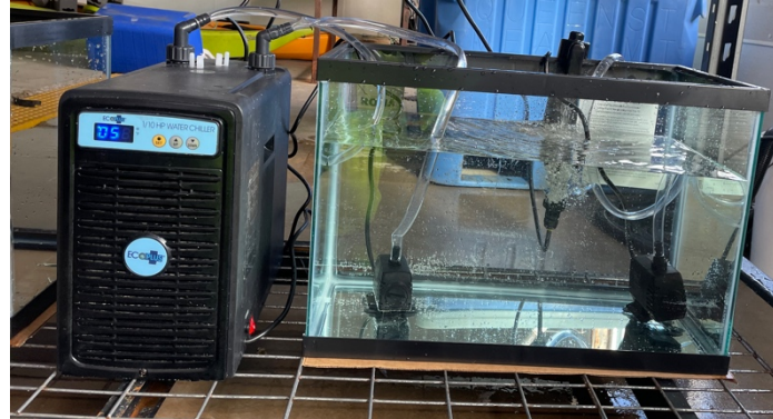
Figure 5 and 6. Seawater is filtered through 5.0, 1.0, and 0.1 micro filters before being placed in the aquarium that is a closed recirculating system with chiller and UV filter on each tank
