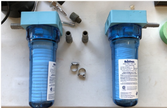
Figure 5 and 6. Seawater is filtered through 5.0, 1.0, and 0.1 micro filters before being placed in the aquarium that is a closed recirculating system with chiller and UV filter on each tank
