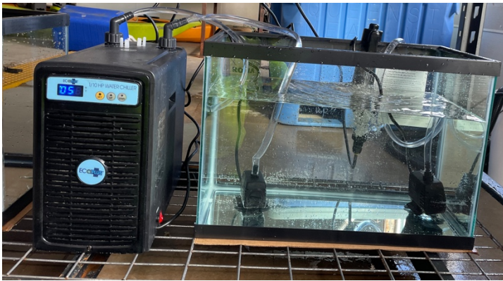
Figures 2, 3, 4 showing 29 gal aquarium set up with chiller and recirculating pump, UV filter and circulating; spools and twine substrate seedlings will grow on in aquarium; seedling growth at 5 weeks and aquarium set up; visible is the two tank system per cohort of seedlings with one of a pair of tanks holding the seedling spools and seawater, pumps etc at time.
