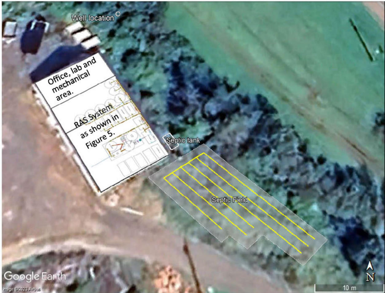
Figure 4: Site layout drawing showing the locations of the well, septic tank and septic field. The septic tank is 5678 L (1500 Gal). The septic field is a standard install with perforated pipe consisting of three lengths of 75', two lengths 50' and one length of 40', as shown in the figure as yellow lines. Note that the well, the septic tank and septic field are already in place. No new construction is needed outside of the building. An enlarged view of the RAS system, as imposed on this scaled image, in white, is shown in Figure 5..
