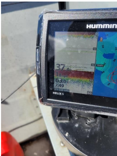
Figure 2. Humminbird fish finder showing arcs just above the lake bottom. Based on angling success, these arcs are likely lake trout investigating the fishing lures.
