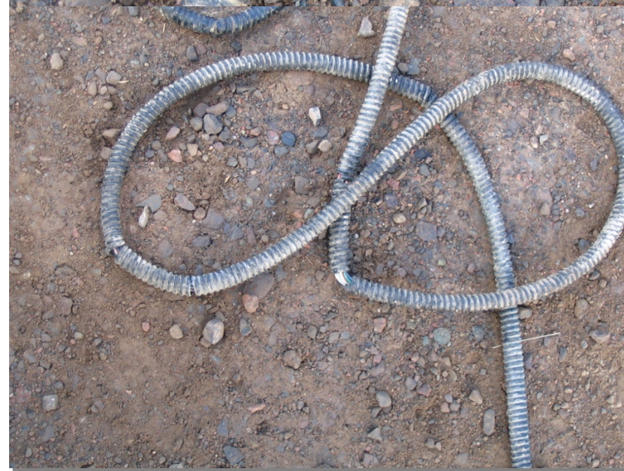
Dangerous - Insulation Cracked
