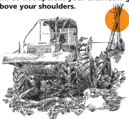
Pulling the tree down with a skidder
