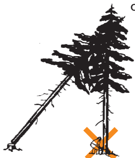
Forest workers should not: — cut down a support tree
