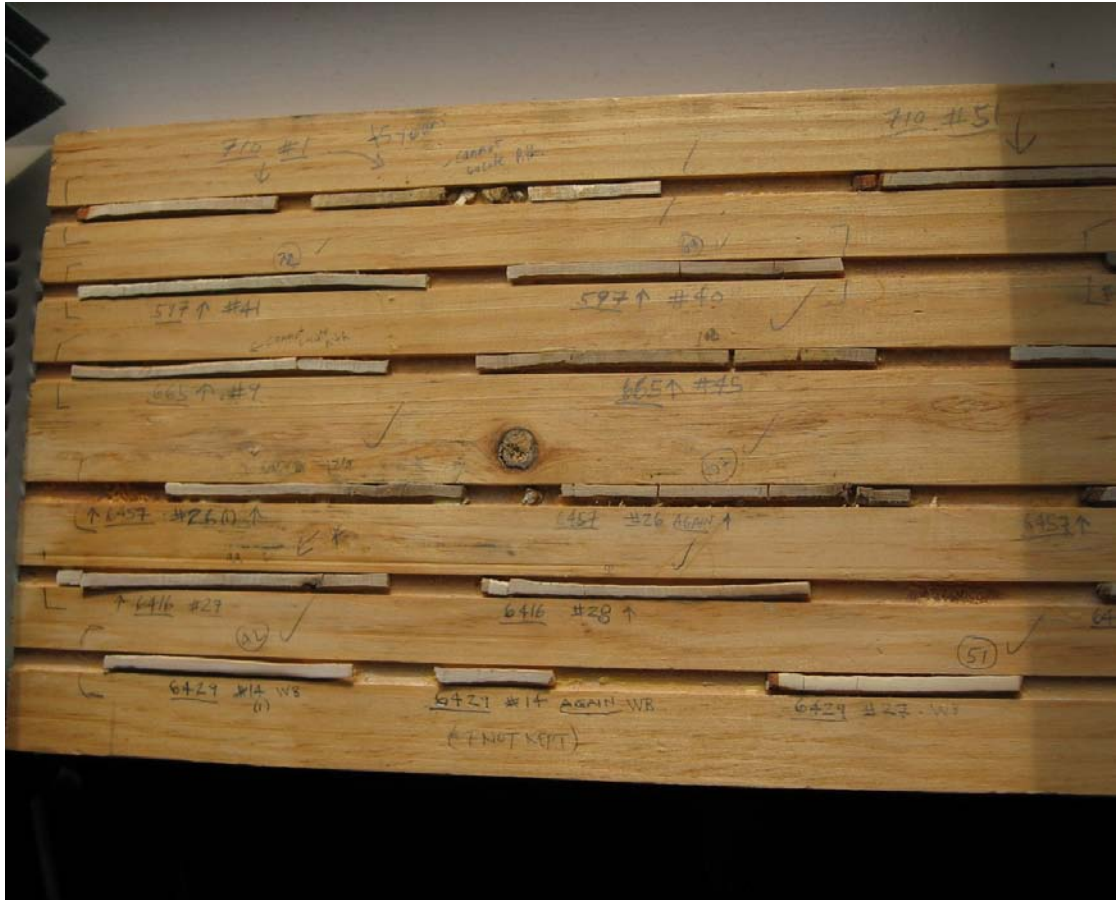
Picture 3. Board with hardwood increment cores. Cores are taken to determine plot age and age of Land Capability trees. Cores that cannot be easily counted in the forest are handled by this method. The cores are glued into the precut grooves, sanded, and then the rings are counted to get the tree age at breast height.
