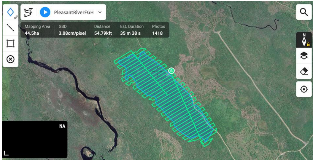
Figure 1. Flight route of the Pleasant River Lake Medium Retention Irregular Shelterwood harvest in Lunenburg County, Nova Scotia. Flight route was created using the DJI Pilot 2 App with a DJI Mavic 3M.
