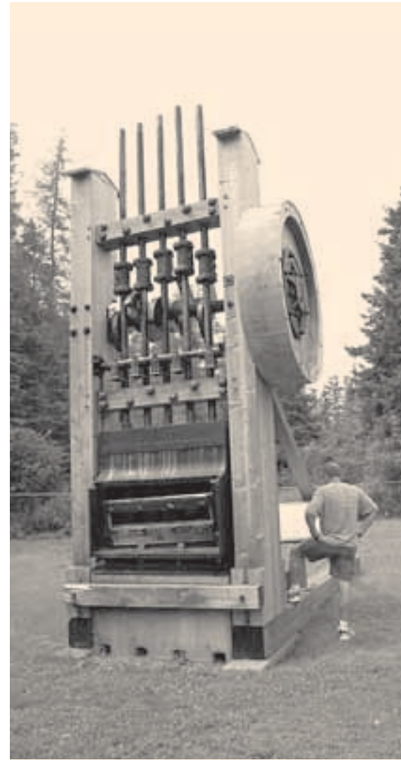
Stamp mills like these were once used to separate gold and heavy metals from the ore.
