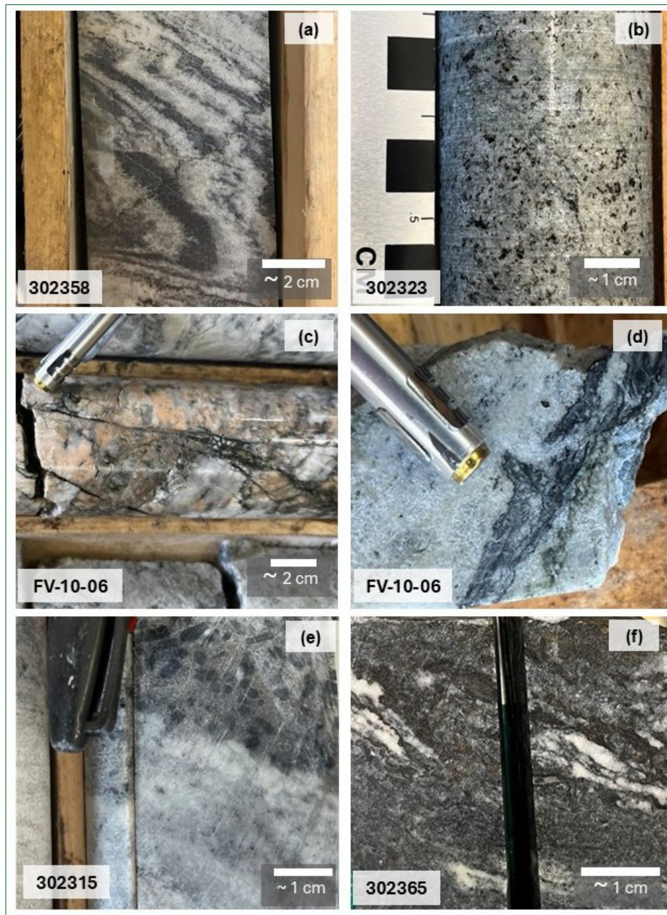
Figure 28. Highlights from 2025 drill core sampling: a) FV-08-04: compressive stress features (z-folds) in grey, banded, marble; b) FV-10-07: grey, marble, local serpentine; patchy graphite (suggested to be the siliceous marble unit “red zone” by Black 2005) in proximity to granitic pegmatite intrusions; c) FV-10-06: feldspar pegmatite (Boisdale Hills Pluton) with graphitic fractures; d) FV-10-06: graphite and calcite development near pegmatite contact (skarn) with marble; e) FV-10-04: light grey, weakly graphitic, tremolite banded marble; f) FV-10-04: black, sheared, pyritic biotite schist (locally graphitic; suggested to be the graphitic biotite gneiss unit “blue zone” by Black, 2005).
