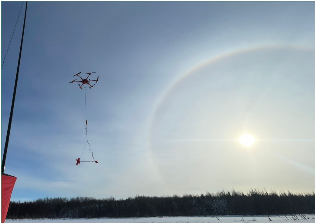
Figure 22. Field photograph of UAV-based geophysical survey operations during the survey period, illustrating the drone platform and suspended sensor payload used for magnetic data collection.
