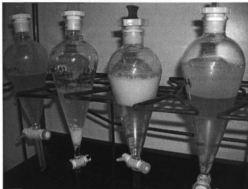
Picture 4.0 Funnel #1, #3 and #4 organic and aqueous after recycled organic is re-loaded with pH 2.8 adjusted leachate solution.
