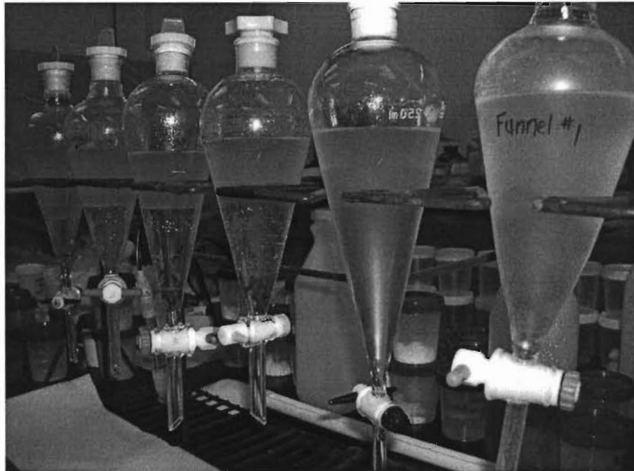
Figure 2. Photograph of the Pb Strip Tests using 0.5 M HNO 3 on Pb Loaded Cyanex 301
