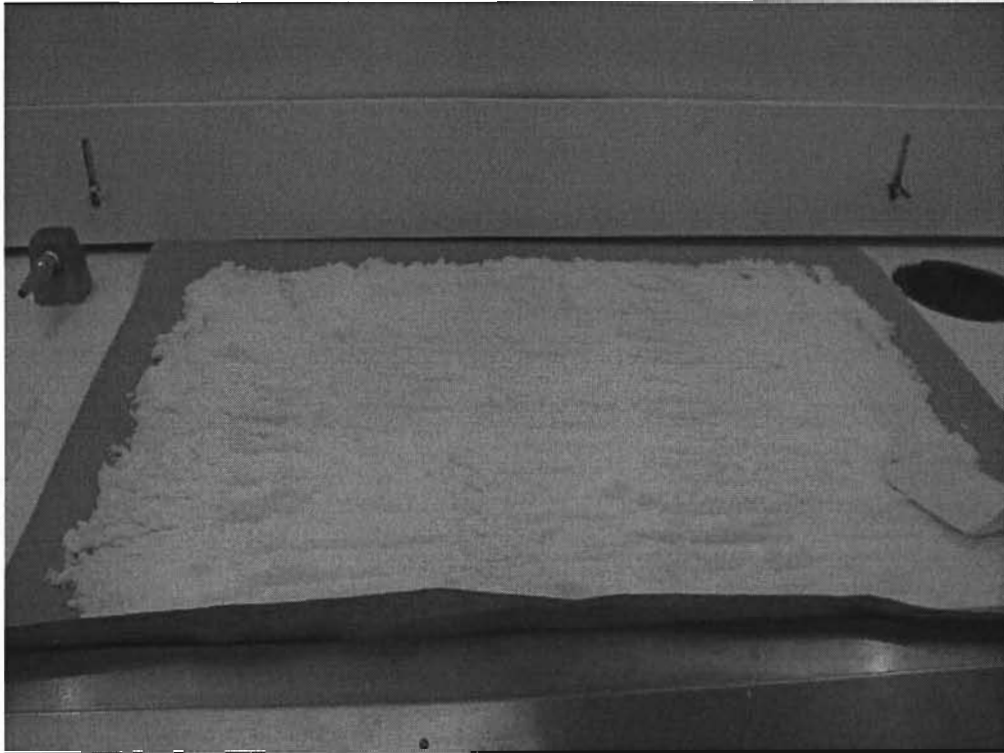
Figure 1: 5-kg \text{Pb}(\text{NO}_3)_2 crystals air drying on craft paper in the fume hood.
