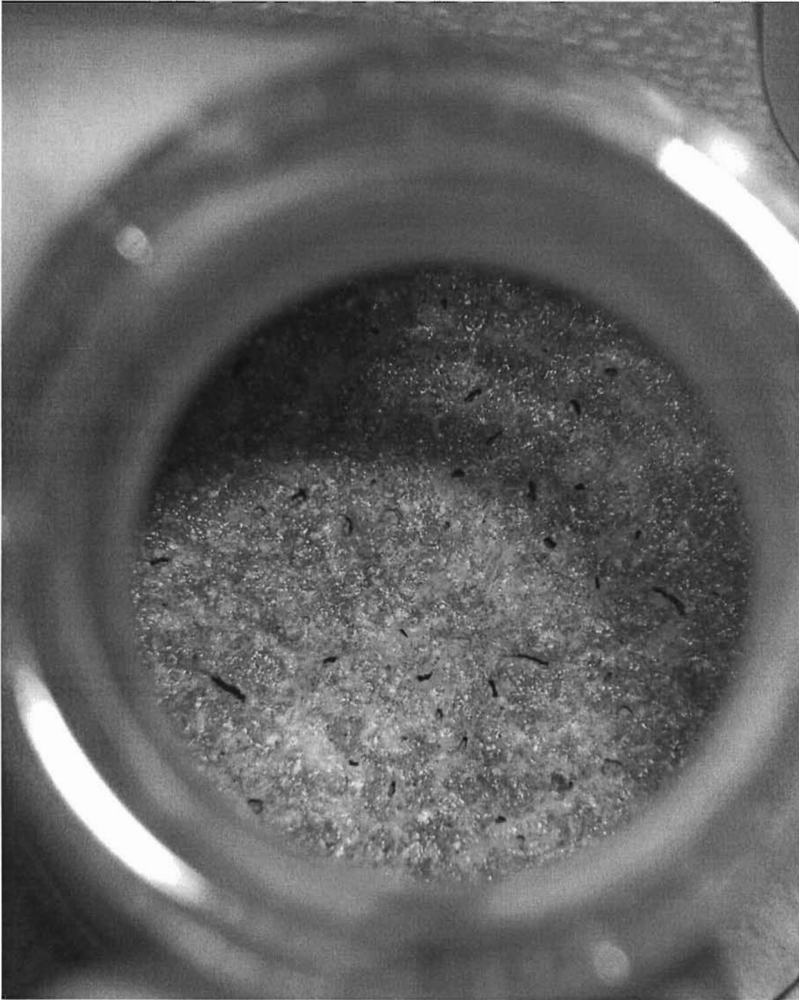
Figure 2. Elemental Sulphur (Yellow Material) Produced in Leach Test D-3
