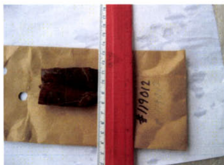
Sample 119012 DL-11 at 124.5 m RHYOLITE small fractures filled with epidote.
