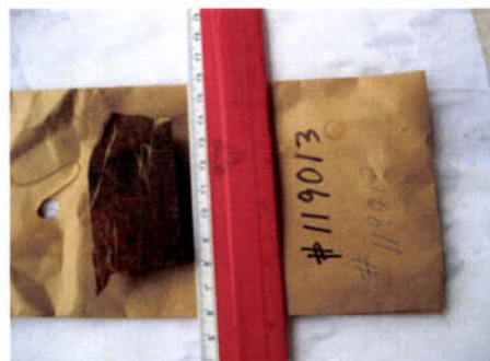
Sample 119013 DL-11 at 124.5 m RHYOLITE small fractures filled with epidote & calcite.
