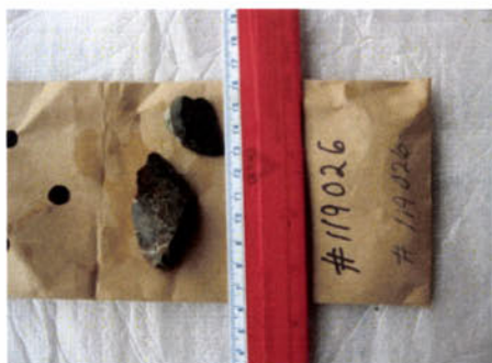
Sample 119026 DL-20 at 57.6 m IGNIMBRITE Chlorite and epidote veins in fractures.
