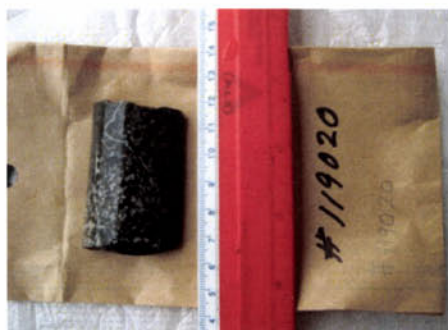
Sample 119020 DL-21 at 63.6 m DIABASE note somewhat coarser phases and filled fractures. (calcite)
