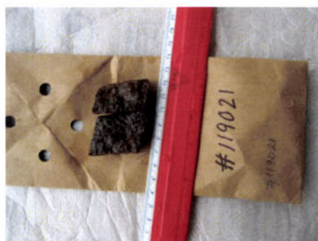
Sample 119021 DL-21 at 68.7 m Granite - pinkish-red becoming pink locally, medium to coarse grained. Composition is variable but approximately 55% - 70% feldspar, 25% - 40% quartz and 10% - 15% hornblende
