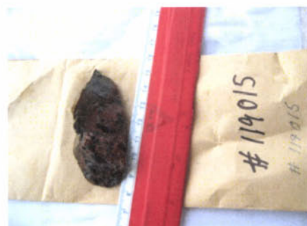
Sample 119015 (DR -04?)DL-21 at 32.5 m Felsic Agglomerate - brick-red altered zones are found associated with strongly fractured zones Note also black chloritic areas?
