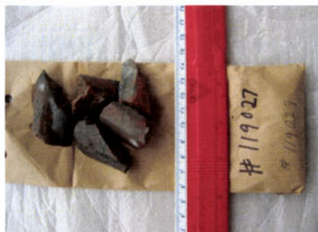
Sample 119027 DL-20 at 115.8 m Rhyolite (Ignimbrite) – light to medium grey, aphanitic and contains abundant angular to sub-angular, pink aphanitic fragments
