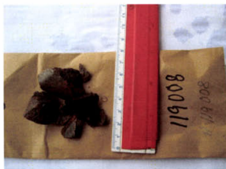
Sample 119008 DL-13 at 162.5 m GRANITE red to pinkish-red, medium to coarse grained and is composed of 20 -30% quartz, up to 80% feldspar and minor amounts of hornblende, magnetite and chlorite
