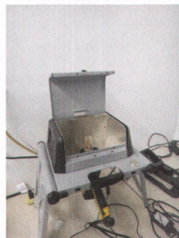
Figure 4-Portable XRF in test stand
