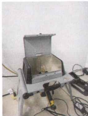
Figure 4-XRF analyzer in test stand
