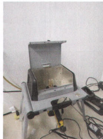
Figure 4-Portable XRF in test stand
