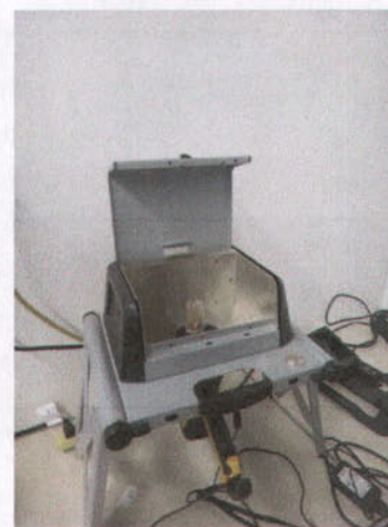
Figure 4-Portable XRF in test stand
