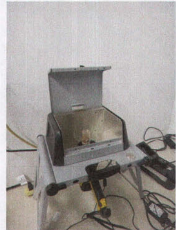
Figure 4-Portable XRF in test stand
