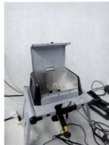
Figure 4-Portable XRF in test stand
