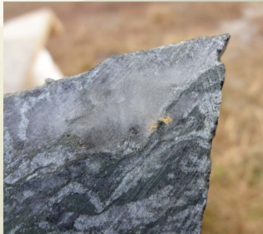
Visible Gold in drill core from Stay Gold's first Drill Hole ~36.5 g/t Au over 0.5m
