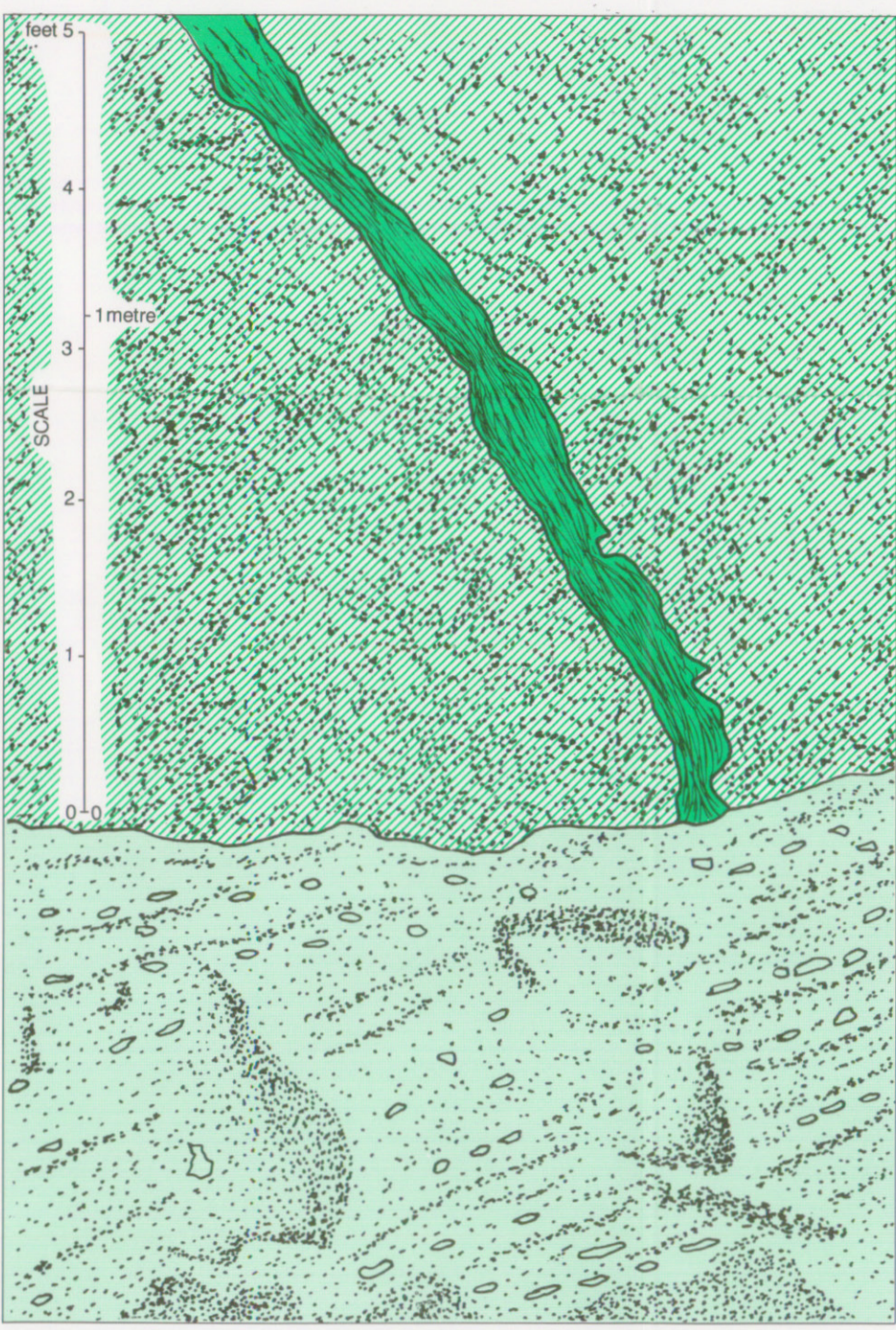
90-2/I - Sketch of a portion of the Shaft Anhydrite Member; detail of C-2 clay marker truncated by grey halite, indicates that the anhydrite unit has been disrupted and is a fragment of an original bed; note flow lineation within the grey halite unit; scale bar is 5 feet; location on 830 level, 2650E and 1550N.
