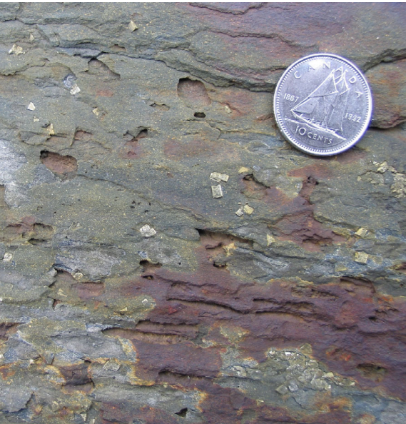
Figure 1. Small, bronze-colored, cubic, pyrite crystals are visibly embedded in this slate. The rusty-colored iron staining indicates ongoing sulphide oxidation and ARD. Photo by G. Payne, NSERN.
