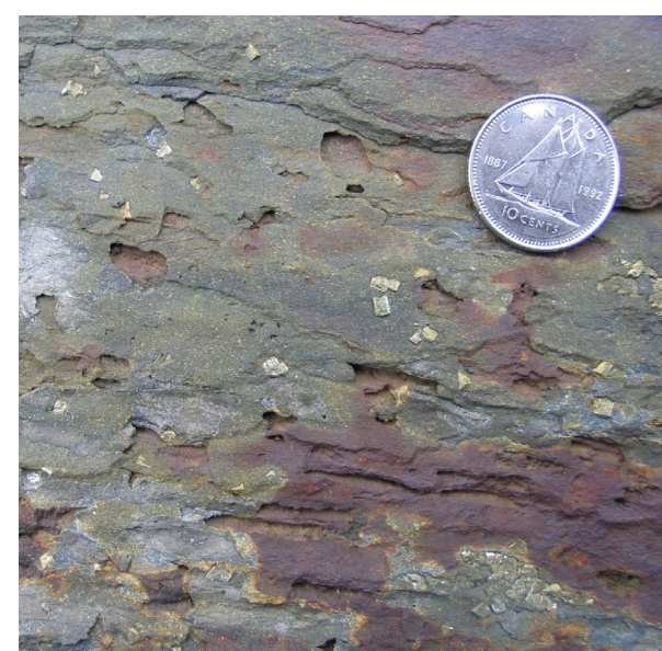
Figure 1. Small, bronze-coloured, cubic, pyrite crystals are visibly embedded in this slate. The rusty-coloured iron staining indicates ongoing sulphide oxidation and ARD (photo by G. Pirnie, NSDNR).
