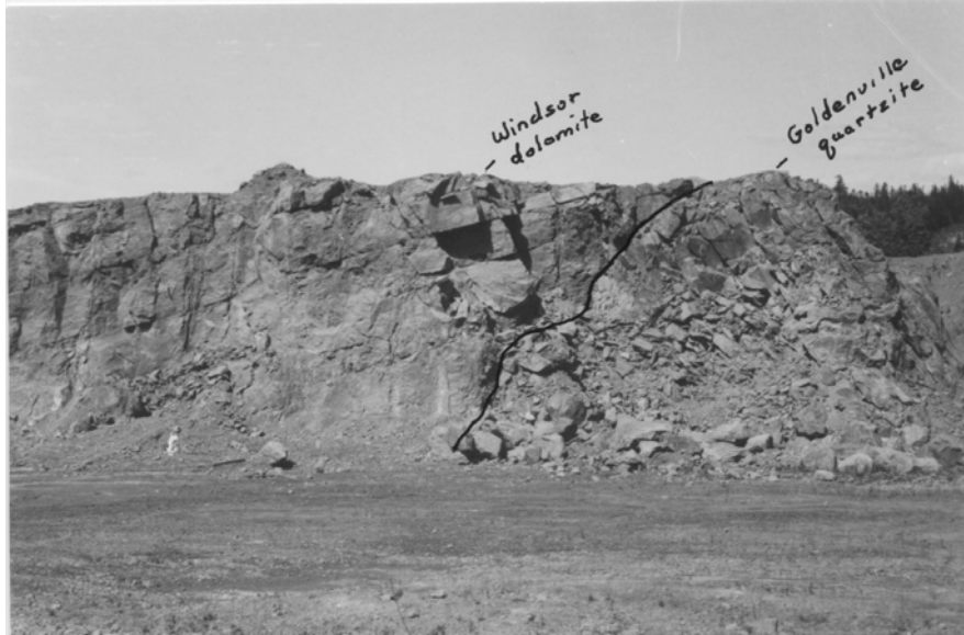
Figure 61. Dolomite can be seen overlapping quartzite in the Upper Musquodoboit dolomite quarry, Halifax County. For location see Figure 60..
