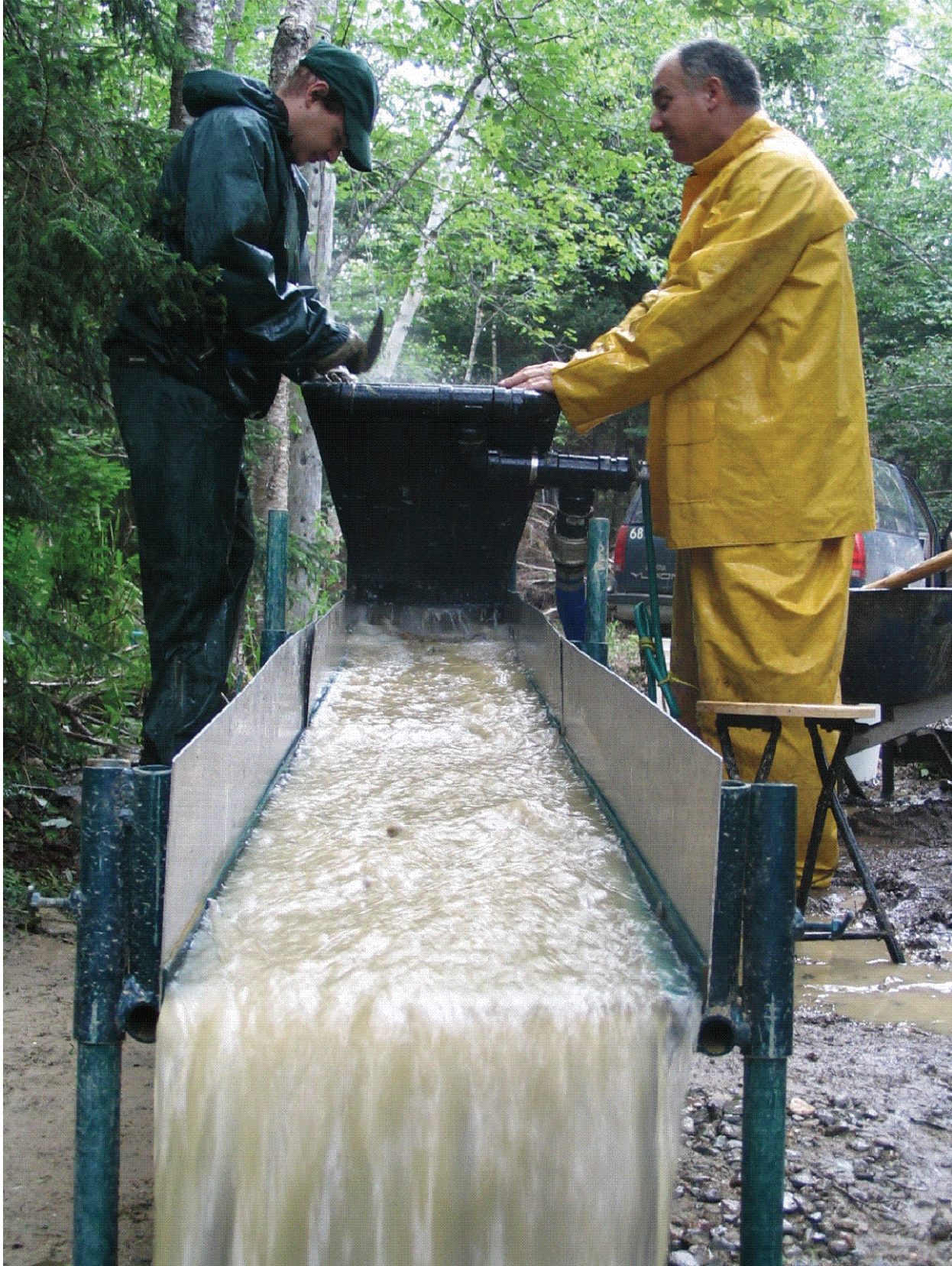
Figure 4. Photo of operation of sluice at Kemptville.
