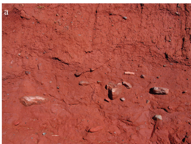
Figure 8a and 8b. Clay-rich till deposits can be used to produce engineered soils for creating impervious barriers or sealing layers in applications such as landfills or dam structures. Figure 8a is a clay-rich till in a shoreline exposure at Burntcoat Head, Hants County. The more distant view of the same exposure in Figure 8b shows that this site has competing interests. Clay-rich soils commonly underlie some of the more productive farmland in the region.
