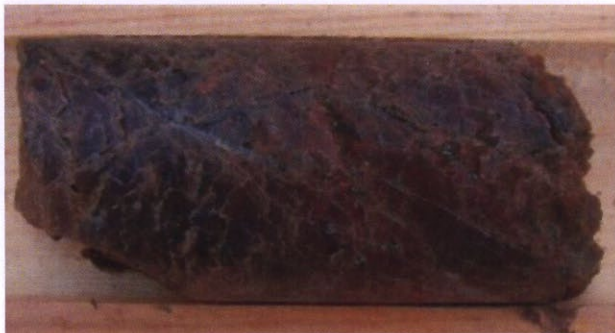
Figure 6. Brecciated and haematized granite with pyrite concentrations along fractures (Drillhole NS05-08-DD1 209m)
