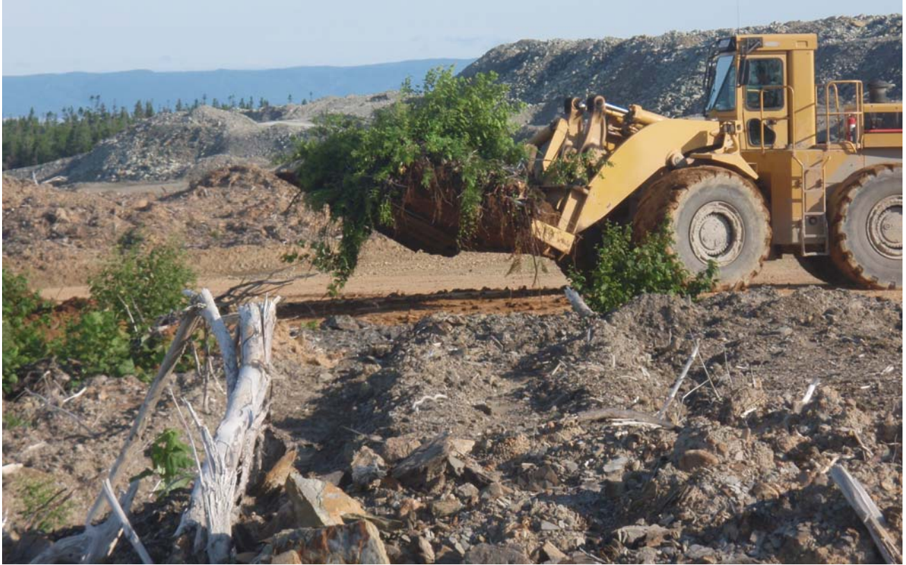
Figure 4. Loader transplanting a 'shrub clump' on a pan-shaped bucket.
