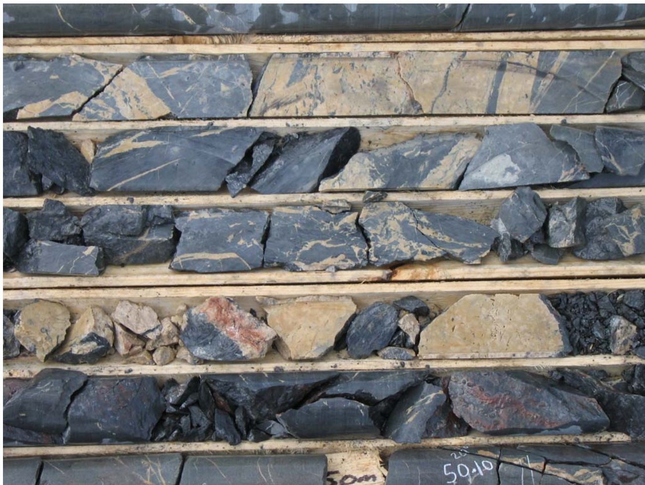
Figure 1. Drill core from Eight Island Lake area, Guysborough County. This is NQ core with a diameter of 47.6 mm.
