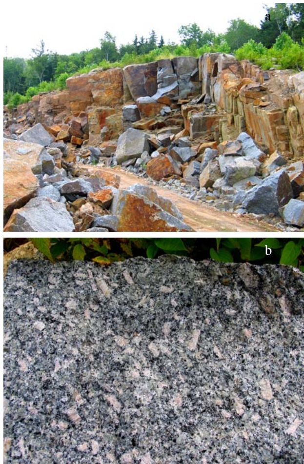
Figure 6a, b. The blasting that created this road cut (Fig. 6a) at Castle Frederick has exposed a mafic porphyry which may have potential for building stone applications. This site is complicated by the presence of sulphides and lead along some of the fracture planes. Note the uncommonly abundant limonite along the joint fractures. Otherwise, the rock is generally fresh in appearance (Fig. 6b). Samples have been taken for cutting and polishing.
