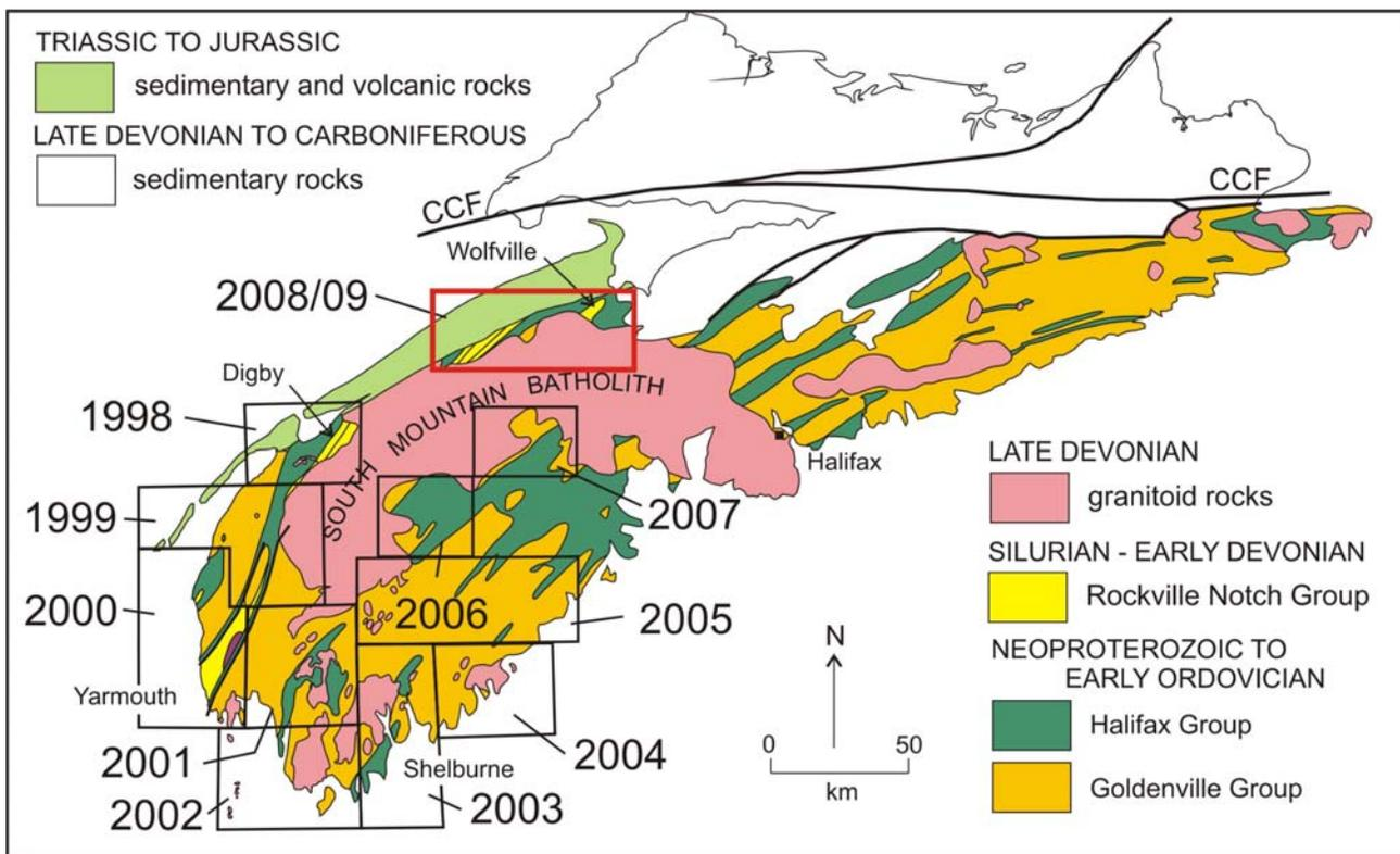
**Figure 1.** Simplified geological map of the Meguma Terrane, Nova Scotia, showing location of the Annapolis Valley map area (red box) in relation to the Southwest Nova and South Shore mapping projects.
