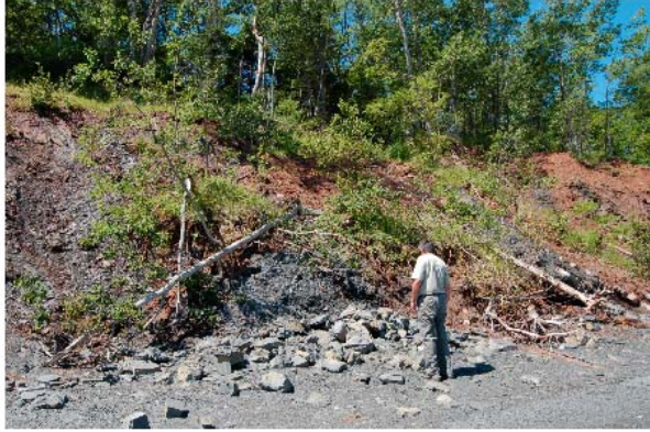
Figure 6. Example of a recent earth flow of till and rock fall (foreground) at Site 1, Figure 2.
