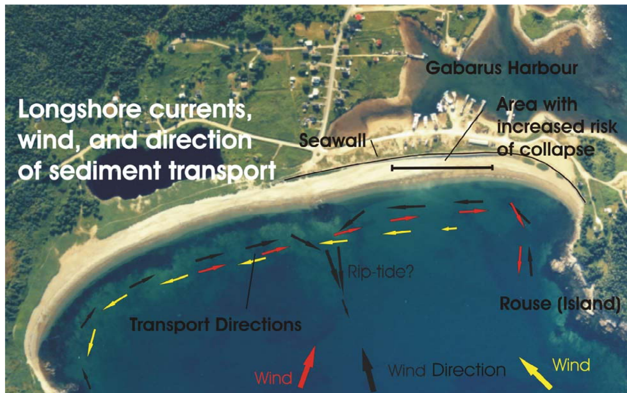
Figure 3. Illustration of general sediment transport in front of the Gabarus Seawall, including the area of the seawall at increased risk of collapse.
