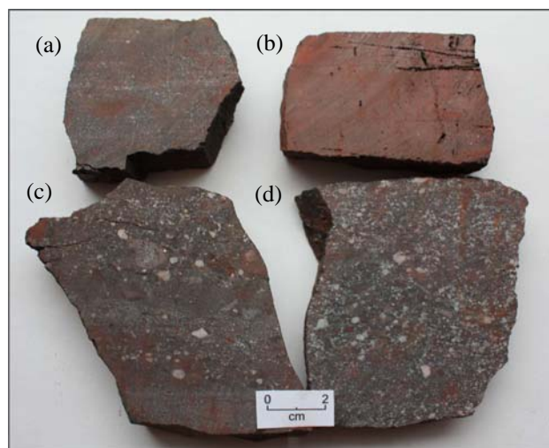
Figure 7. Rock slabs displaying various textures in the ironstone beds. (a, c, and d) Samples from the Iron Brook Group. (b) Sample from the French River Formation (Arisaig Group).
