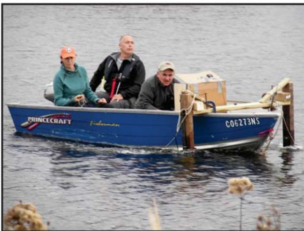
**Figure 5.** The author and two collaborators from the Geological Survey of Canada (Atlantic Division) conducting seismic and sidescan sonar surveys in Irish Vale Pond. Instruments are mounted on wooden frame across bow of NSDNR boat.
