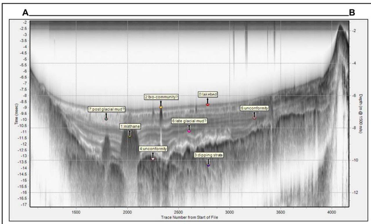
**Figure 6.** Initial interpretation of seismic surveying in Amaguadees Pond. Location of line A-B is shown in Figure 4. Labels on figure (initial interpretation): 0. lakebed; 1. shallow methane; 2. oyster bioherm; 3. dipping strata below lowest unconformity; 4. lowest unconformity; 5. another unconformity; 6. late glacial mud; 7. post-glacial mud.
