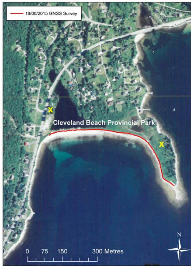
Figure 2. Cleveland Beach Provincial Park shoreline in St. Margarets Bay, Halifax County. Red line is the GNSS survey, which followed the vegetation line and/or greatest break in slope, separating the beach from the leading edge of coastal erosion. Yellow x symbols show locations of the two erosion control point markers for Cleveland Beach Provincial Park (to be installed at a
