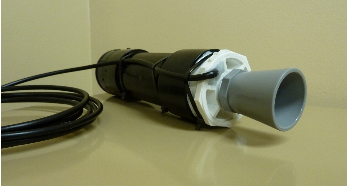
Figure 6. External antenna cable inserted through case bottom and sealed with silicon.
