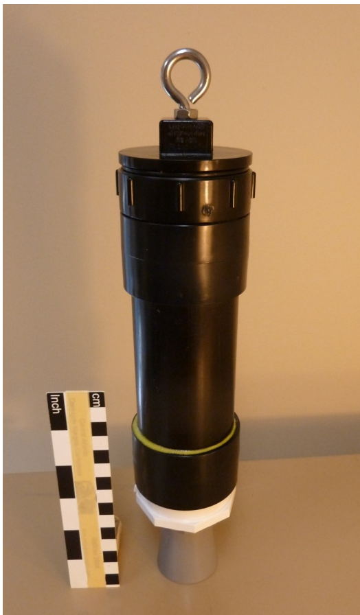
Figure 1. External view of meter. Dimensions: 320 mm long (tip to tip), 50 mm diameter.
