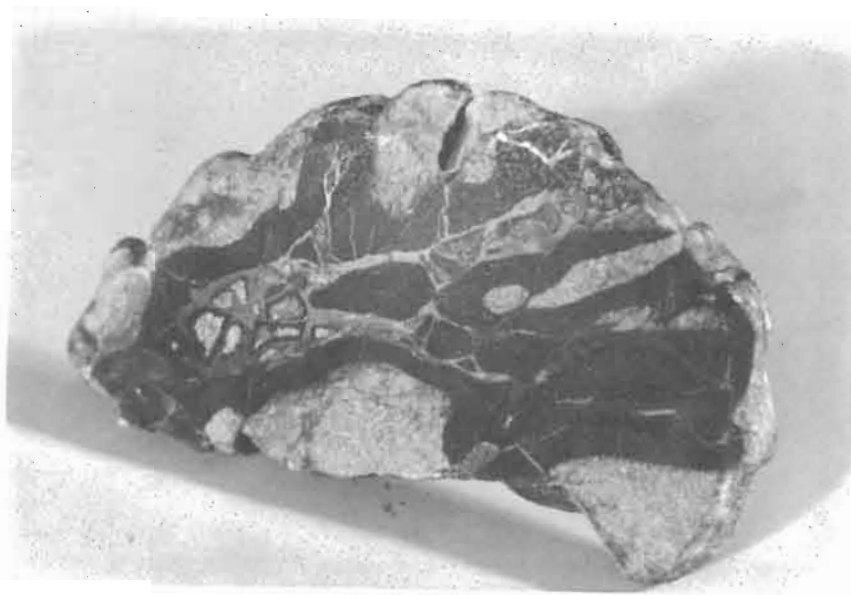
Figure V Network of manganite veinlets (light grey) surrounded by area of partial replacement by pyrolusite of Cheverie quartzose sandstone. Sturgis Mine, Walton, Hants County. Locality No. 6
