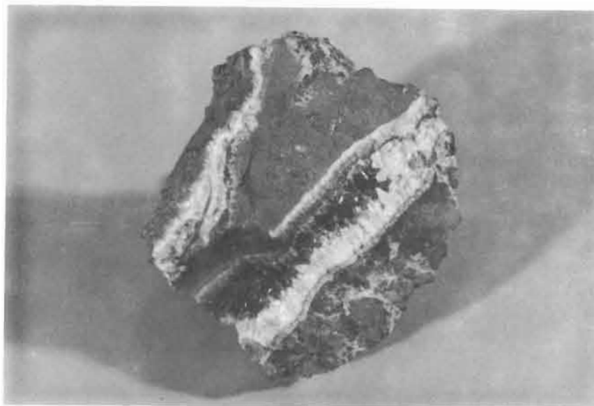
Figure IX Vein of white dog tooth spar with interior lined with fibrous pyrolusite crystals in Pembroke limestone conglomerate, Faulkner property, Hants County. Locality No. 21
