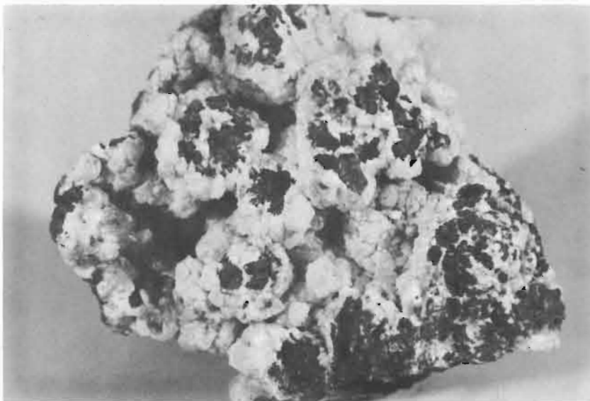
Figure IV Nodules of pyrolusite enclosed by calcite. Dresser Minerals Mine dump, Walton, Hants County. Locality No. 8
