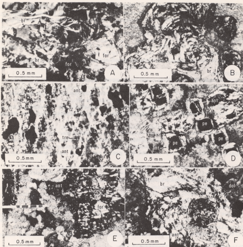
Plate 1. Photomicrographs showing the textural relationships of antigorite and brucite. A, Alteration of forsterite to brucite. B, Alteration of antigorite to brucite. C, Alteration of tremolite to antigorite. D, Alteration of periclase to antigorite. E, Alteration of forsterite to antigorite. F, Alteration of dolomite to brucite and antigorite. for, forsterite; dol, dolomite; ant, antigorite; br, brucite; pe, periclase.
