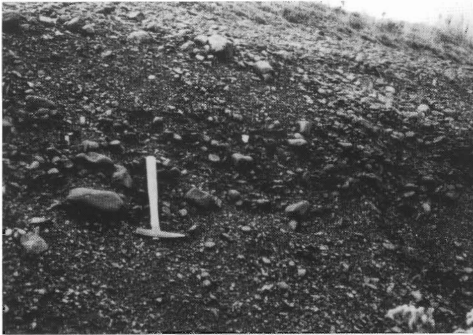
Figure 22. Conglomerate residuum at Eatonville, Cumberland County. Materials are very similar to gravel near the surface. This pit was used to produce Class C gravel for highway upgrading.
