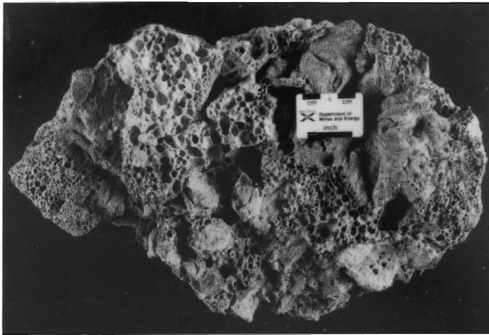
Figure 33. Sample of slag taken from Londonderry, Colchester County. Note honeycomb texture of the material.
