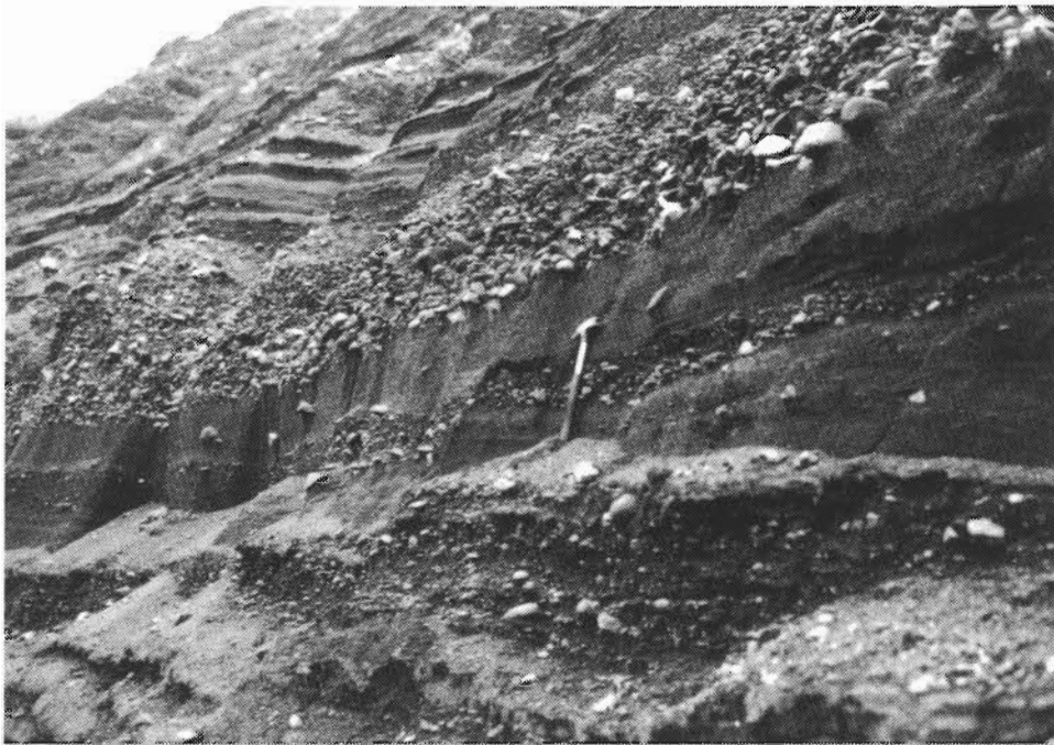
Figure 11. Pit exposure of well sorted, well stratified ice contact deposit (kame delta) at Halfway River Station, Cumberland County.
